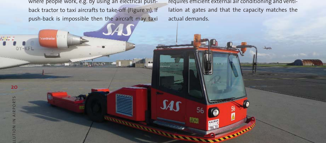
Figure 11: Electrical push-back tractors eliminate local emissions
